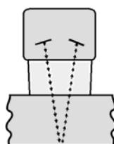
**Dual Element Transducer showing V-path of signal**
