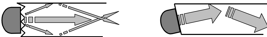
Figure 2 Rough and angled transducer contact
