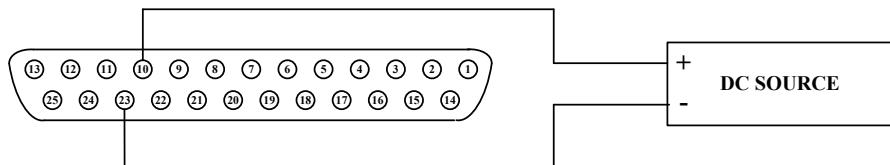
You may access **MENU 6-SPECIAL TEST FUNC** → **2. EXTERNAL CONTROL** to choose the input voltage range at [EXTERN PROGRAM] to [10 V / 10 K] for 0 – 10V and [ 5 V / 5 K] for 0 – 5V.
