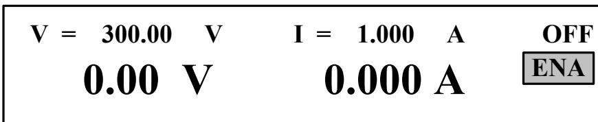
When pin 1 and 14 are **shorted**, the output **On/Off** button is enabled.
