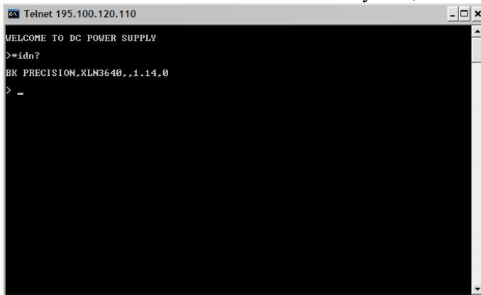
A screenshot of a Windows Telnet window titled "Telnet 195.100.120.110". The window displays the text "WELCOME TO DC POWER SUPPLY", a prompt ">\*idn?", and a response "BK PRECISION,XLN3640,,1.14,0". The window has standard window controls (minimize, maximize, close) and a vertical scroll bar on the right.
