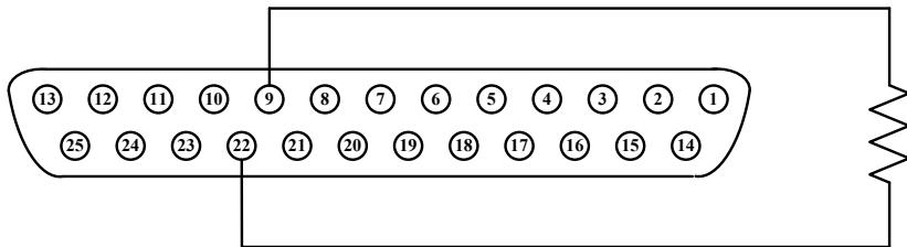
You may access **MENU 6-SPECIAL TEST FUNC** → **2. EXTERNAL CONTROL** to choose the input resistance range at [EXTERN PROGRAM] to [10 V / 10 K] for 0 – 10 kΩ and [ 5 V / 5 K] for 0 – 5 kΩ.
