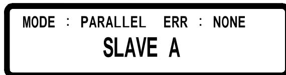
Once the Master and Slave settings are done, users can then operate the Master only to set up the combined output voltage and current of the complete system.
