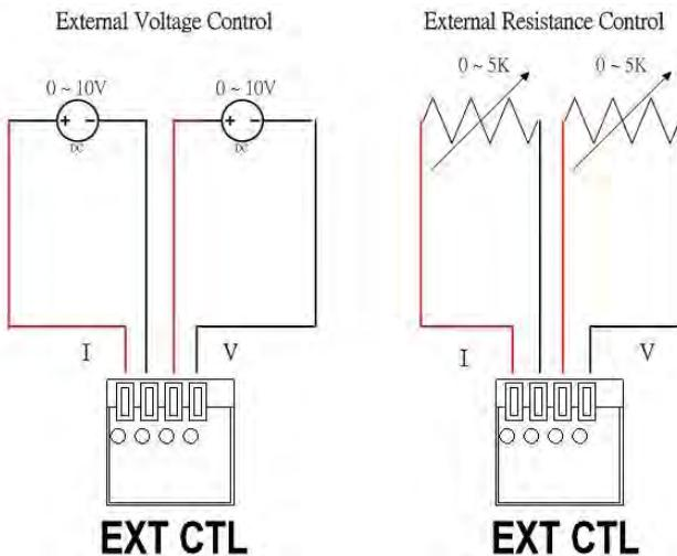
The external voltage control or external resistance control can be set in the “system setting” screen. Since the external control circuit uses a 12bit D/A converter for 0 - 36 V for XLN3640 (or 0 - 60 V for XLN6024 or 0 - 80 V for XLN8018 or 0 - 100 V for XLN10014) output voltage and 0 - 40A for
