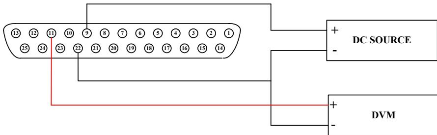
You may access **MENU 6-SPECIAL TEST FUNC** → **2. EXTERNAL CONTROL** to choose the voltage monitor output range of Pin 11 at [EXTERN MONITOR= ] to [10V] for 0 – 10 V (as shown in figure below) and [5V] for 0 – 5V.
