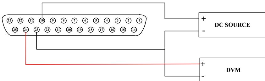
You may access **MENU 6-SPECIAL TEST FUNC** → **2. EXTERNAL CONTROL** to choose the current monitor output range of Pin 24 at **[EXTERN MONITOR]** to **[10 V]** for 0 – 10 V (as shown in figure below) and **[5V]** for 0 – 5V.
