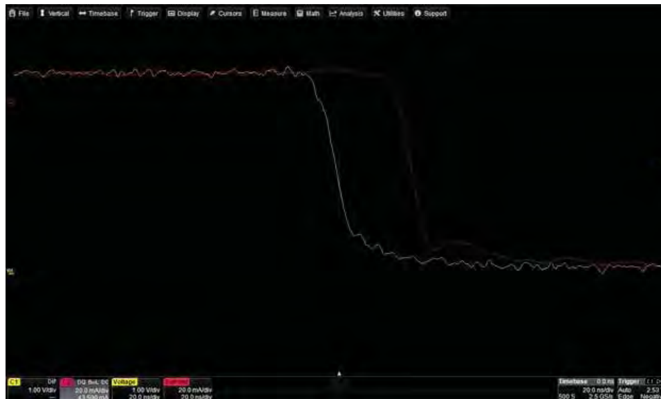
Falling edge of voltage and current traces before deskew adjustment.
