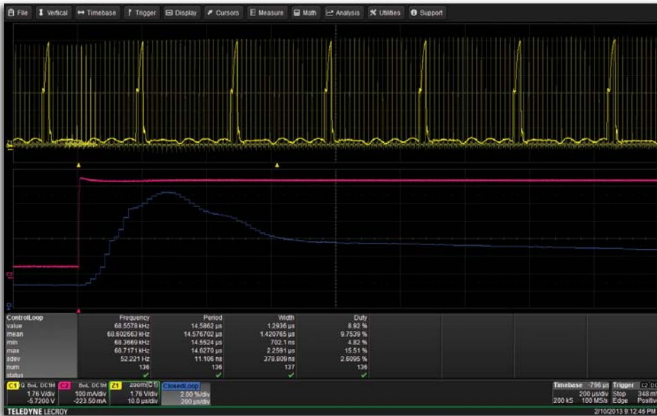
Triggered by the step change in load current (red trace), the gate-drive modulated signal (yellow traces) is captured, the closed-loop, time-domain response of the feedback loop (blue trace) is displayed, confirming loop performance.
