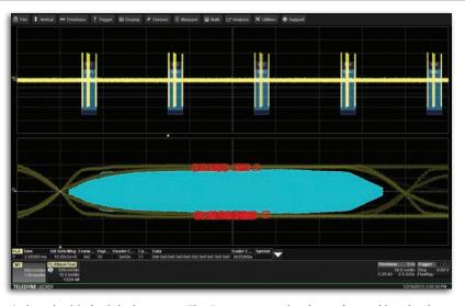
Gain valuable insight into your FlexRay communications channel by viewing eye diagrams, physical layer measurements and decoded protocol data at one time.
