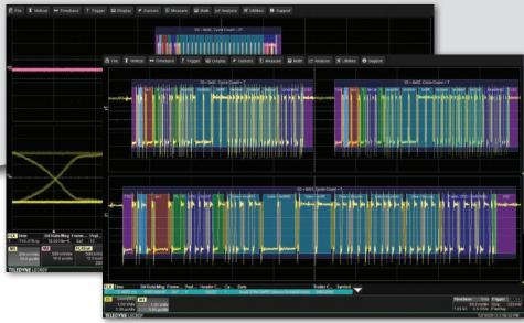
Trigger on Static or Dynamic Slot IDs and FlexRay Symbols, apply a color-coded, easy-to-understand decode over your FlexRay signal, perform automatic eye diagram mask testing and make physical layer timing measurements.
