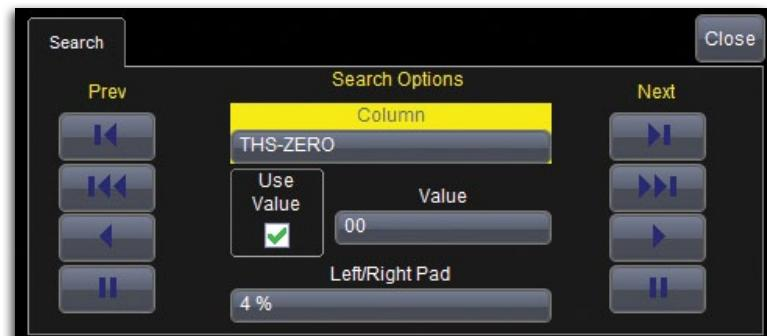
Quickly and easily search for a signal type of interest. Choose from 28 criteria to quickly pinpoint an area of interest, zoom in, and analyze. Use previous and next controls to find the next instance for quick and easy debug.
