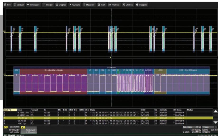
With CAN and CAN FD trigger and decode the oscilloscope becomes the ideal tool for debugging CAN controllers, busses and systems. Identify and isolate specific CAN frames with ID, Remote and Error frame triggering. Decoding CAN signals provides tremendous insight into activity on the bus and measurement tools enable fast analysis of bus performance.
