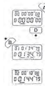
Depress D to select the operating mode. The 'CHRONO' indicator is shown. Depress A to start.
