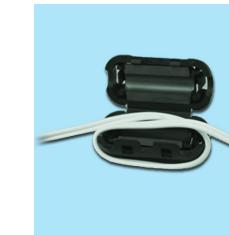
Loop the right end of the cable under the suppressor and back up again laying the cable along the center of the suppressor.
