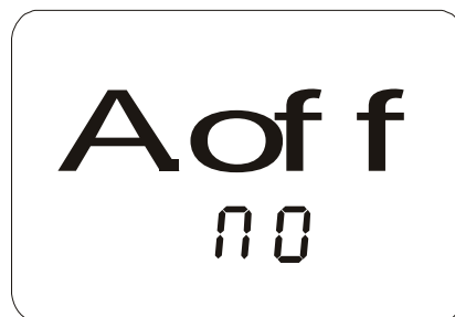
Figure 9: Disabling the auto off function
