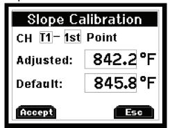
Use the ▲ or ▼ keys to adjust the value to match known temperature standard. Press F1 to accept. Then move to second temperature point using the ▲ or ▼ keys and repeat.
