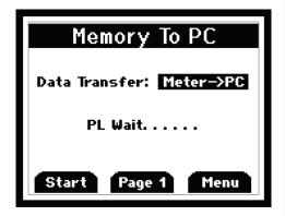
Once the USB connection is established, press the Start button to download data from Meter to PC using HyperTerminal.
