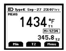
On initial start-up, the meter will display the measured value for input one in the primary display and for input two in the secondary display.
