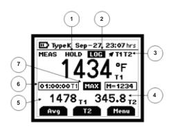
The dot matrix display features a large primary display, smaller secondary displays for channel info or Min/Max/ Avg readings, and helpful annunciators for added measurement data.
