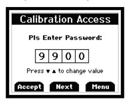
Before you go into the calibration mode, you must enter the password. Press F2 to change to the next digit. (Default Password is 9900)
