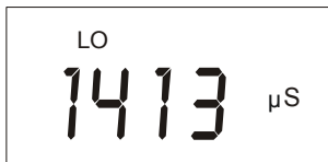
"LO" Battery Condition
