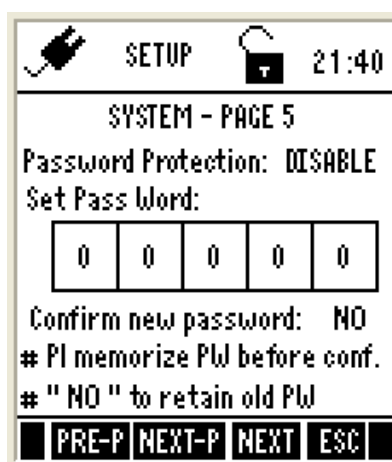
Figure 6: System Settings Page 5 – Password Protection
