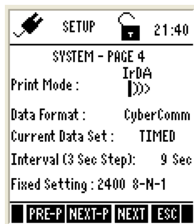
Figure 5: System Settings Page 4 – Wireless Serial Data Communication
