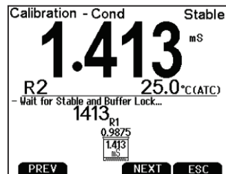
Before and after a one-point automatic conductivity calibration with 1.413 mS
