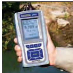
Rubber boot protects meter in rugged environments
