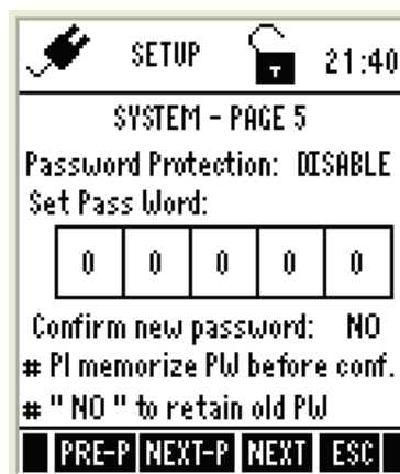
Figure 6: System Settings Page 5 – Password Protection
