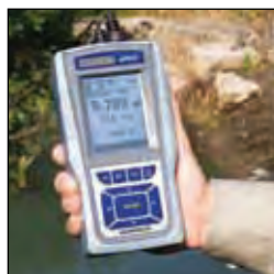
Rubber boot protects meter in rugged environments
