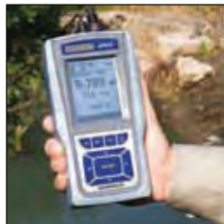
Rubber boot protects meter in rugged environments
