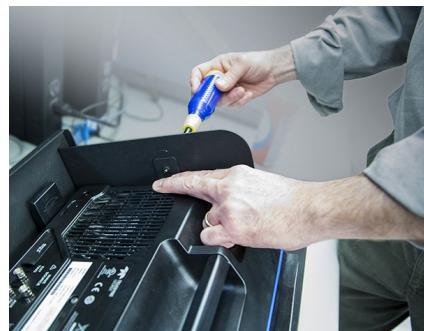
6. Place the oscilloscope on the base plate flush with the face plate. The screen should be fully visible and the front bezel should extend slightly past the face plate when seated properly.
