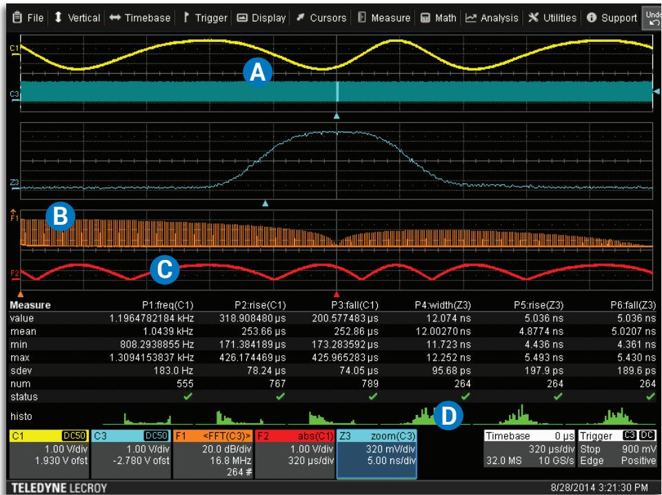
**A** With 10 GS/s and 16 Mpts per channel every detail of a signal will be captured and displayed. In 4 channel operation 1.6ms of data can be captured at full sample rate, in 2 channel mode, 3.2ms, to ensure no detail or anomaly is missed.
