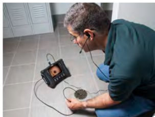
Record video with audio during pipe inspections
