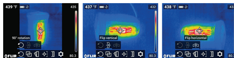
Figure 7.2 Selecting 90° Rotation or Vertical/Horizontal Flip.
