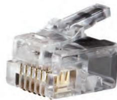
Klein's data and telephone plugs are professional-grade and deliver consistent, reliable performance. Our thick 50 micro-inch gold plating on contacts prevent erosion and extended connector life. The three-pronged contacts provide more reliable connections with solid and stranded wire. The plug is housed in a durable resin with a spring clip. Expect a sure connection each and every time.
