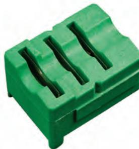
Designed for use with Klein's Radial Strippers. Three levels of blades strip RG58, RG59 and RG62 coax cable. Pre-set cutting blades save time and provide precise cutting. The cartridge is made from glass filled polycarbonate for increased strength and durability.
