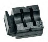
Designed for use with Klein's Radial Strippers. Two levels of blades strip RG59, RG6 and RG6 QS coaxial cable. Pre-set cutting blades for precise and accurate stripping. Durable high-carbon steel cutting blades are ground and honed for long life. Patented "V" notch eliminates scoring of the center conductor.
