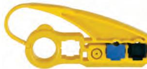
The Klein Tools Dual-Cartridge Radial Stripper is ideal for high-volume, multiple-type cable preparation environments. To facilitate left or right-handed operations, cartridges snap in from both sides. The cutting blades are a durable high-carbon steel cartridge, ground and honed for long life.
