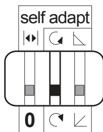
Figure 6. DIP Switch Set for Clockwise Rotation.
