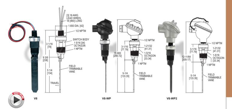
The Series V8 Flotect® Vane Operated Flow Switches are ideal for protecting unattended equipment from damage or loss of production. This Series is available for installation in a 1 to 6" pipe with operating pressures are up to 150 psig (10 bar) and temperatures to 212°F (100°C).
