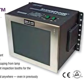
The **UV-400A** features a concentrated-beam reflector designed to assure the highest concentrated UV-A intensity available. It has a peak steady-state UV-A intensity of 8,000 µW/cm² within the lamp's center area, measured at 15 inches (38 cm). The lamp irradiates an area as large as 16" x 10" (41 cm x 25 cm), producing a nominal steady-state UV-A irradiance of not less than 2,000 µW/cm<sup>2</sup>.
