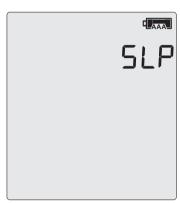
A hibernated logger cannot be reactivated via the buttons - it must be reconfigured with LogTag® Analyzer.
