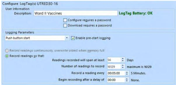
Adjust the settings as required. For detailed information about each parameter please read the section about  $Configuring \ a \ LogTag^{\ B}$  for  $logTag^{\ B}$  Analyzer's User Guide or press F1 for help.
