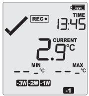
The logger will now track new min/max values. A min/max reset mark will be recorded in the logged data. As soon as the next reading is taken, both minimum and maximum values will be shown again. You will be able to see on the PDF and in the summary in LogTag<sup>®</sup> Analyzer when the min/max values were cleared, but you will not be able to review previous min/max values on screen once they have been cleared.
