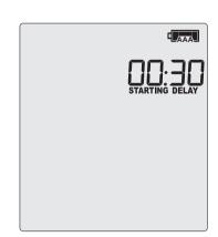
The timer can be cancelled and the logger reset to **READY**. While **STARTING** and **DELAY** are shown, press and hold the **START/CLEAR/STOP** button. **STOPPED** will now show. Release the button when **STARTING** disappears.
