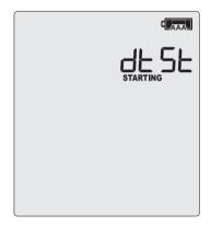
The UTRED30-16 will perform a Connection Test as soon as the recording has started. To check the connection before the start time is reached, you can initiate the connection test yourself. Please refer to Testing your wireless and network connection (on page 1).
