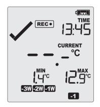
If the sensor was disconnected for a complete day, the minimum and maximum statistics for that day will show on the display and --.- in the list.
