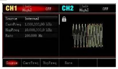
2) Set Hop Frequency After step 1), press HopFreq, enter 800 by numeric keypad, and select parameter unit Hz.
