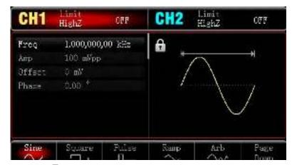
Press | Amp | to set amplitude, enter 1 by numeric keypad, and select parameter unit | Vpp |. Press Duty to set duty ratio, enter 50 (default) by numeric keypad, and select parameter unit %.
