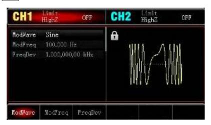
2) Set Modulation Signal Parameter and Waveform After step 1), press | ModWave  $| \rightarrow |$  Square | to select square wave as modulation waveform. Press MadFreq, enter 2 by numeric keypad, and select parameter unit kHz.
