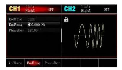
3) Set Waveform and Parameter of Carrier Wave Signal Press | Wave | → | Sine | to select sine wave (default) as carrier waveform.
