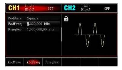
3) Set Waveform and Parameters of Carrier Wave Signal
