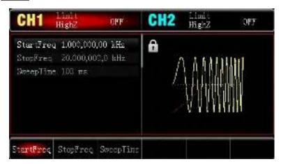
Press | StartFreq | / | StopFreq |, enter 1 by numeric keypad, and select the parameter unit | kHz |. The start frequency is 1kHz by default.
