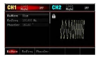
2) Set Modulation Signal Parameter After step 1), press | ModFreq |, enter 200 by numeric keypad, and select parameter unit | Hz |.
