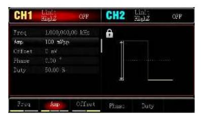
Press | Freq | to set the frequency, enter 10 by numeric keypad, and select the parameter unit | kHz |. Press Amp to set the amplitude, enter 200 by numeric keypad, and select the parameter unit mVpp. Press Duty to set the duty ratio, enter 45 by numeric keypad, and select the parameter unit %. As shown below:
