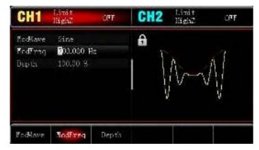
3) Set Waveform and Parameter of Carrier Wave Signal Press | Wave | → | Square | to select the square wave as carrier waveform (default to sine wave).
