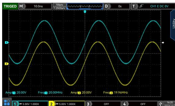
Large output under the high frequency: double channel with full amplitude output of 20 Vpp can be output under the frequency of 20 MHz.
