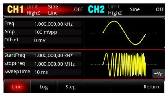
Three sweep frequency modes: "Line", "Log" and "Step". Three trigger sources: "Internal", "External" and "Manual".
