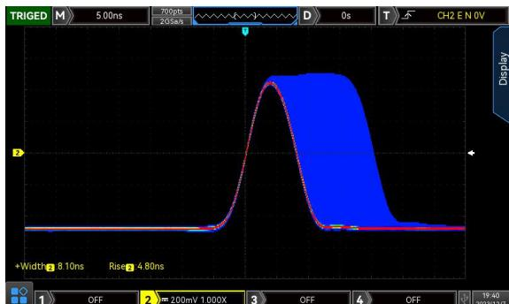
The new generation of wide dynamic high precision edge time adjustable pulse wave has a minimum pulse width of 8 ns. The pulse width can be fine adjusted and the minimum step is 100 ps. In addition, it can produce higher harmonic component, which has the feature of a dedicated pulse generator. The edge time can be set to a minimum of 5 ns independently.
