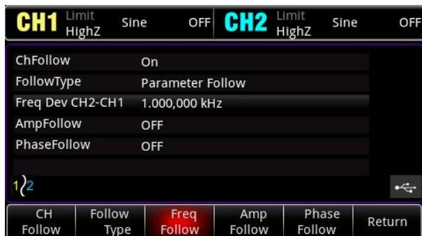
Channel tracking simplifies the operation of dual channels. The phase, amplitude and frequency of both channels can be controlled by a single parameter, making it easy to create deviation or tracking signals.
