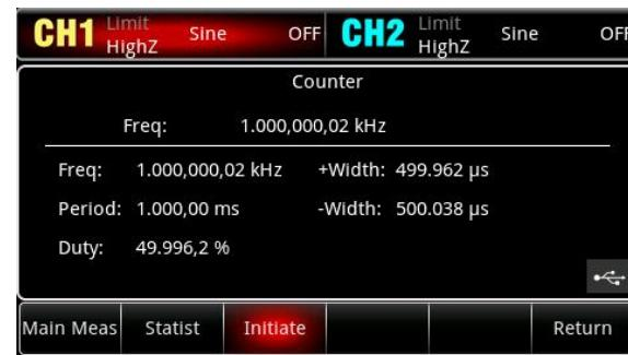
The high precision hardware frequency counter can measure the frequency range of 100 mHz~200 MHz.
