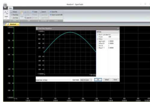
The arbitrary waveform editor has diversified generating method. The arbitrary waveform can be generated by insert the standard waveform or freely drawing.
