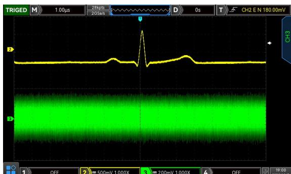
Channel merging can be realized with SUM or channel stacking functions, generating signals with adjustable signal-to-noise ratios and dual-tone multi-frequency signals. Up to four signals can be summed and coupled on two channels, and SUM enables the output of two-tone or multi-tone signals.
