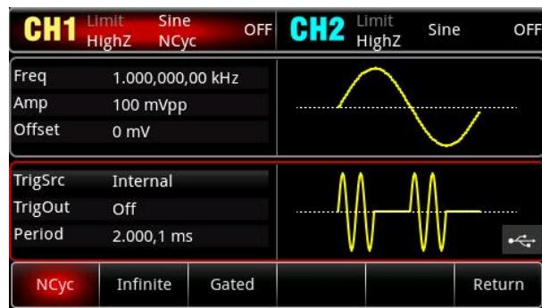
Three types of bursts: "N cycle", "Infinite" and "Gate". Three trigger sources: "Internal", "External" and "Manual".
