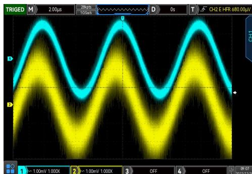
A small signal superimposed with a large DC results in a lower output noise and a higher SNR.
