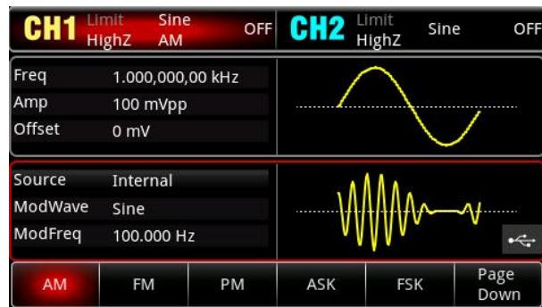
Modulation output (15 types): AM, FM, PM, DSB-AM, ASK, FSK, PSK, 3FSK, 4FSK, BPSK, QPSK, OSK, SUM, QAM and PWM.
