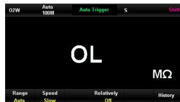
Figure 3-3 Reading of short-circuit test leads
