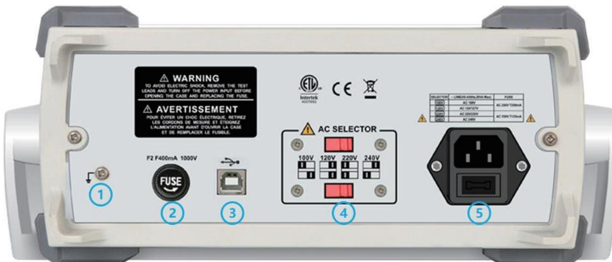
①1 Grounding ②2 Fuse socket ③3 USB interface ④4 AC voltage selector ⑤5 Power supply interface
