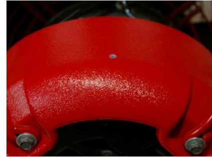
Figure 17: Pressure sensor on the fan motor casing.
