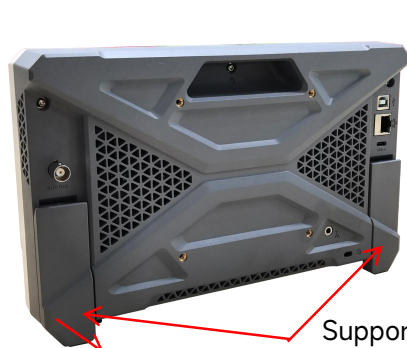
Unfold the supporting feet
