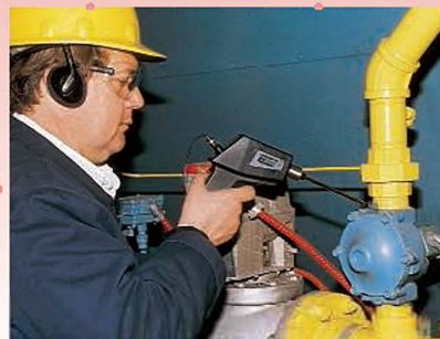
Ultraprobe 100 testing pump valve leaks
