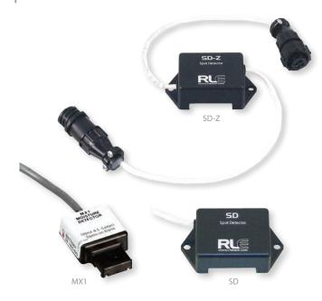
SD, SD-R01, SD-Z and MX1 Spot Detectors detect conductive fluids at a single point for the most economical way to detect fluids in small, confined areas. These devices are commonly used in small rooms and in air-conditioning drip pans. Use only with SC conductive fluid leak detection cables.
