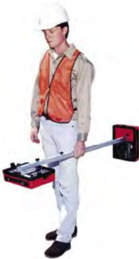
The Model TW-6 "Two-Box" metal detector finds underground pipes, cables, manhole covers, vaults, valve boxes and other metallic objects.
