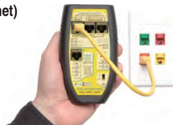
The lights quickly tell you if the device is a hub/switch
