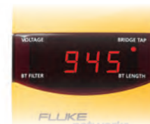
Bridge tap found at 945 feet /288 metres
