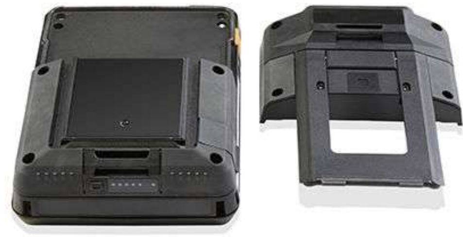
Figure 2-7: Trex unit with the communication module removed
