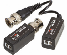
HDB-VSTPT2 5MP Video Balun, 1 with Pigtail, 1 Without CVI 720P 450m, 1080P 250m, TVI 720P/1080P 250m AHD 720P 320m, 1080P 250m
