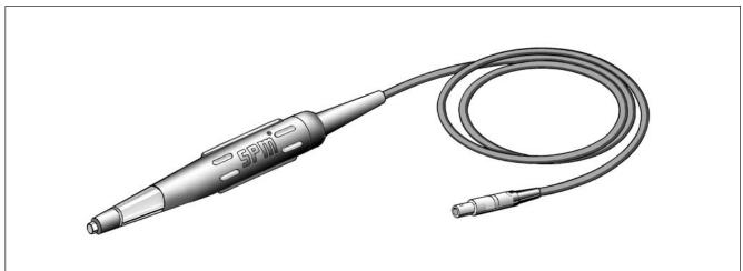
TRA-73 is a hand-held probe, which is used together with BearingChecker. The probe is directionally sensitive and must be held aligned against the bearing and not deviate from this direction by more than  $\pm 5^{\circ}$ . The probe tip is spring loaded and moves within a sleeve made of chloroprene rubber (neoprene) and tolerates 110 °C (230 °F).
