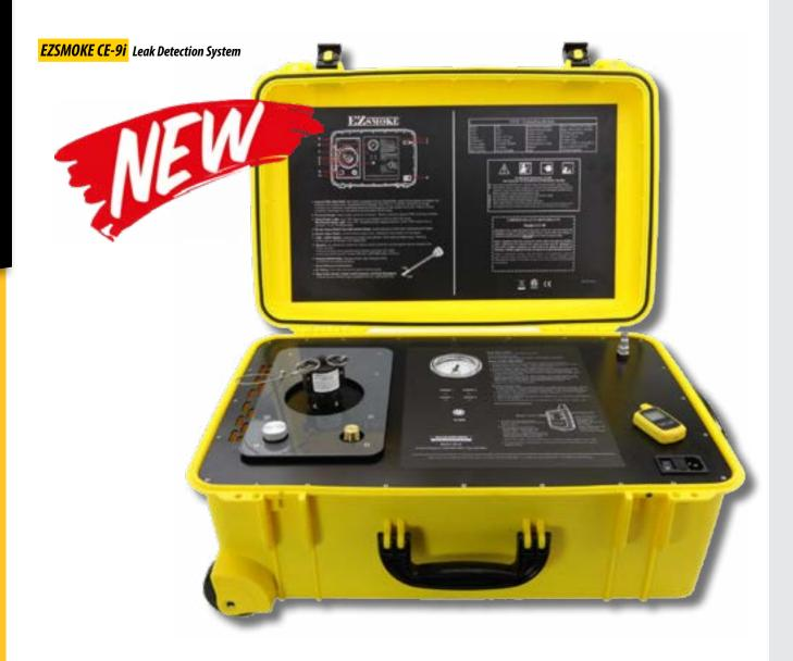
EZSMOKE allows a technician to use low pressure, non-toxic smoke, with a pleasant lemon scent and UV dye, to quickly locate annoying sewer gas leaks that are often difficult and time consuming to find in cuts, cracks, fractures, punctures, porosity or unsealed fittings inside or outside residential or commercial buildings.
