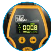
Displays neutral to ground voltage
