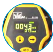
Trips GFCI at 6mA or 30mA
