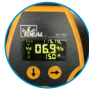
Displays Voltage Drop at 12, 15 & 20 Amps
