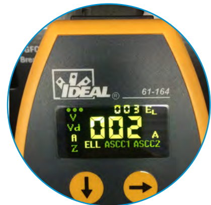
Estimated Load on Line in Amps
