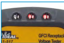
Red Lights Indicate Incorrect Wiring
