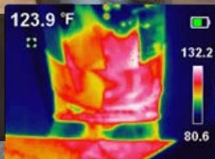
Locate insulation gap to improve energy efficiency
