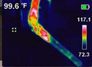
Find compromised seal on ductwork joint to eliminate heat loss
