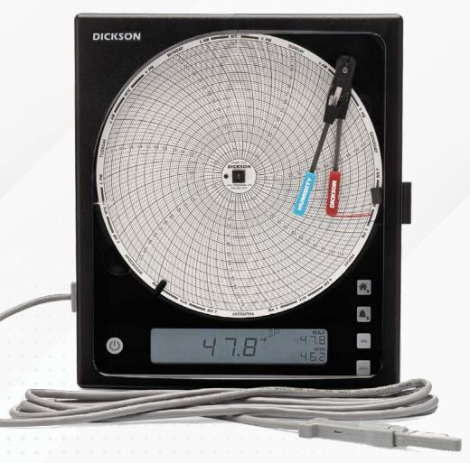
8" (203mm) chart recorders offer the largest resolution out of any chart recorders. All chart recorders feature a large 8" chart and user-selectable recording time-frames and ranges. These units are compatible with Dickson's Replaceable Sensors™, making calibrating your chart recorder easier than ever.
