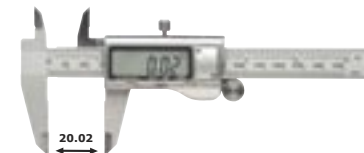
Differential method measurement (application of zero setting)
